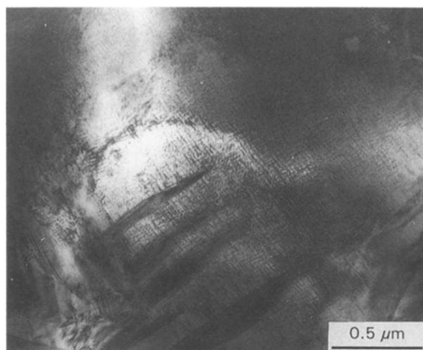
Figure 3 Electron micrograph of a rapidly quenched specimen showing tweed structure.
